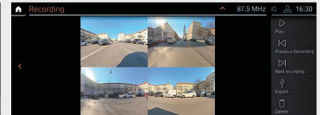
□ The BMW Drive Recorder\* allows you to record a video from the vehicle environment and play the video on the central Control Display or via USB export also on your CE device. Important vehicle information such as speed and GPS position are stored synchronously with the video. The Drive Recorder has two sub-functions, the Event Recorder and the Crash Recorder.
