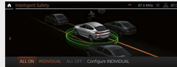
□ Driving Assistant Professional<sup>3</sup>\* offers optimum comfort and safety during critical or monotonous traffic situations. Apart from the contents of the Driving Assistant, it also includes Steering and Lane Control Assistant with extended functions, Lane Change and Emergency Stop Assistant and Lane Keeping Assistant with active side collision protection.
