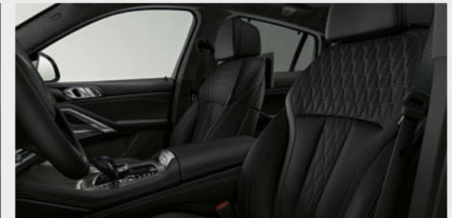
□ The comfort seats for driver and front passenger include active headrests and can be electrically adjusted in various ways. The top part of the backrest, the backrest width, thigh support and headrest height can be individually adjusted. The equipment package range also includes the lumbar support and memory function for the driver.
