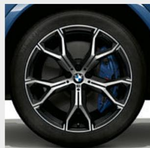
□ 21" M light alloy wheels Y-spoke style 741 M Bicolour Orbit Grey with mixed tyres, gloss-lathed, front 9.5J x 21 with 275/40 R21 tyres, rear 10.5J x 21 with 315/35 R21 tyres.<sup>2,3,6</sup>
