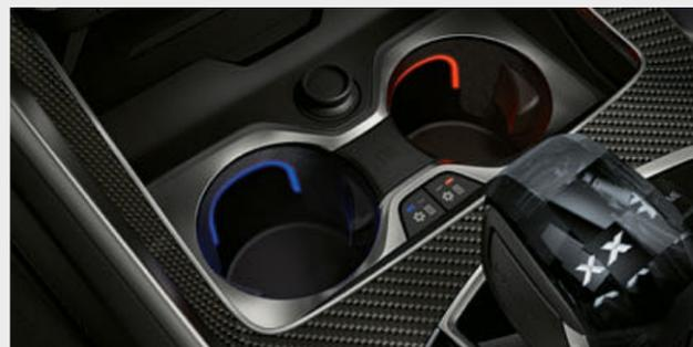
□ The temperature-controlled cupholders in the centre console can individually cool or keep stored beverages warm. The temperature control is activated via buttons on the left and right. The ambient lighting also indicates the function (blue for cooling or red for heating).
