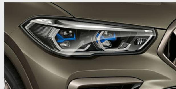
□ In laser high-beam mode, BMW Laserlight in a unique X design illuminates a range of up to 500 m, nearly twice as far as that of conventional headlights. Better visibility in the dark significantly increases safety. The blue X signature and the "BMW Laser" lettering underline the vehicle's technological standards.
