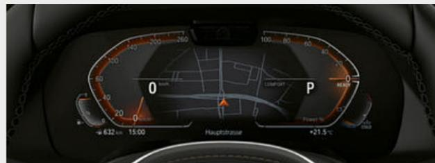
■ The BMW Live Cockpit Professional with navigation function<sup>1</sup> includes two high-quality displays consisting of a high-resolution 12.3" Control Display that can be operated by touch and a fully digital 12.3" instrument display.
