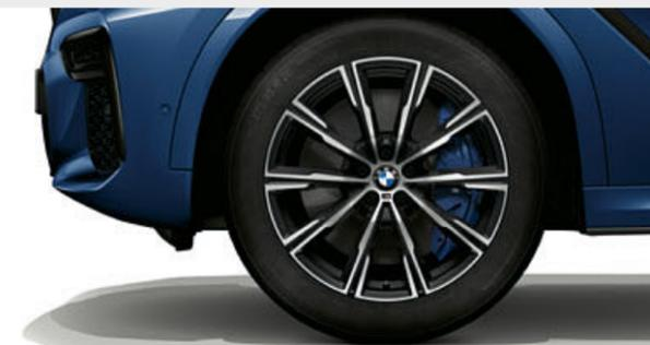
■ 20" M light alloy wheels Star-spoke style 740 M Bicolour Orbit Grey with mixed tyres and runflat tyres, gloss-lathed, front 9J x 20 with 275/45 R20 tyres, rear 10.5J x 20 with 305/40 R20 tyres.
