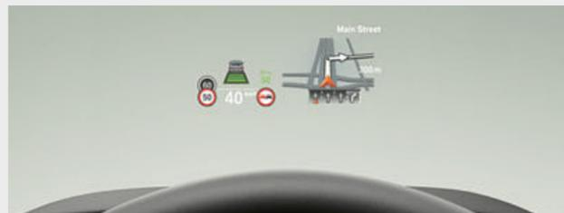
□ The full-colour BMW Head-Up Display<sup>2</sup> projects all information relevant to the journey directly into your field of vision, allowing you to fully concentrate on driving. Information such as the current speed, navigation directions, speed limit info including no-overtaking indicator, along with telephone and entertainment lists are displayed, depending on the equipment.
